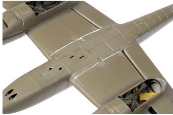
While the putty was still pliable, the remainder was used to smooth a tiny step at the lower wing joins.
