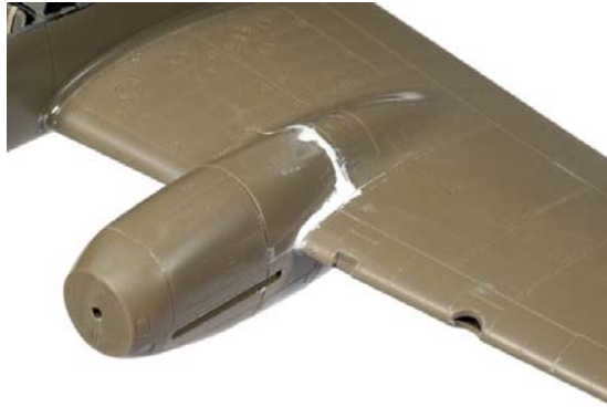
The step outboard of the engine nacelle was also filled with Milliput.
