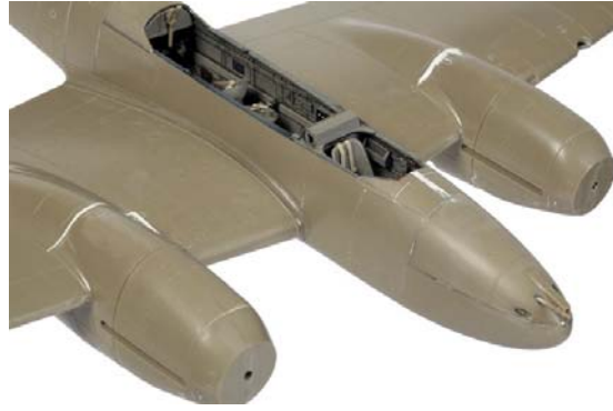
Milliput, a two-part epoxy putty, was used to address the engine nacelle gaps and steps, plus a few smaller alignment issues. Masking tape was used to ensure the Milliput did not spread beyond the area requiring filling.
