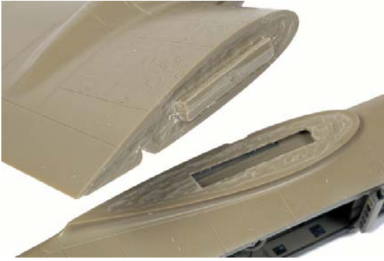
The large flat mating surfaces of the wing and the fuselage at the wing root were ground back using a round dental burr in my Dremel motor tool. This ensured a gap-free fit.
